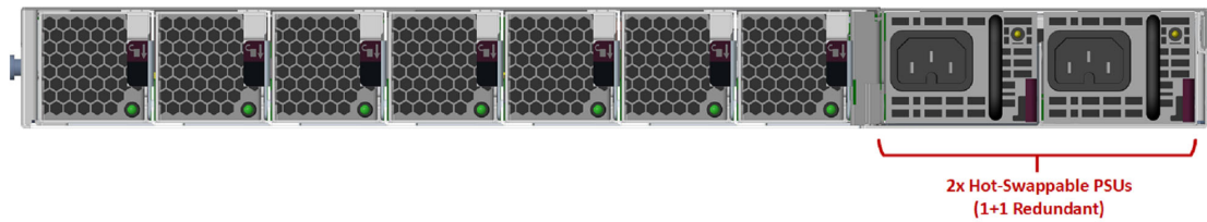
Figure 3. TippingPoint TPS TXE devices - back panel location of power supplies (9200TXE shown)
