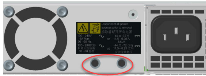
Figure 6. TippingPoint TPS 5600TXE devices - DC grounding screw holes to accept the lug connector attached to ground
