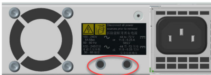
FIGURE 6-8. Ground screw location for 5600TXE devices
