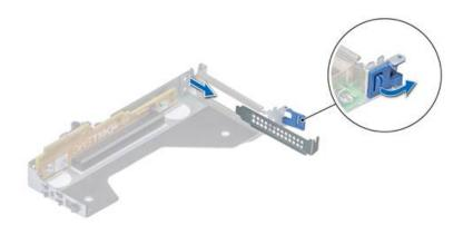
**d.** Align the card with the server's PCI-e slot, push the card in firmly until the card is connected, then close the card retention latch.
