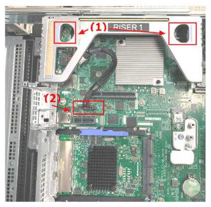
**c.** Open the card retention latch and remove the PCI slot cover of an empty PCI-e slot
