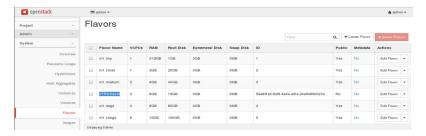
e. Click the down arrow next to **Edit Flavor** to set the hw:vif\_multiqueue\_enabled metadata as True for the flavor. This update is necessary for images of CPUs with three or more cores.
