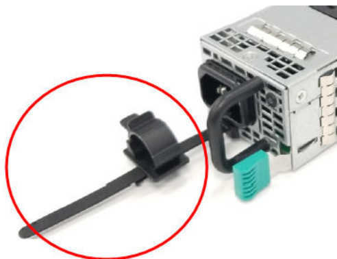
FIGURE 8-4. Retention clip for TXE power modules
