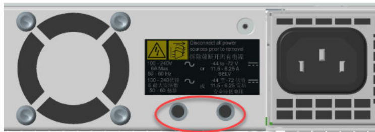
FIGURE 8-8. Ground screw location for 5600TXE devices
