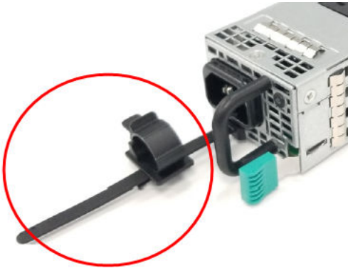
FIGURE 8-3. Retention clip for TXE power modules
